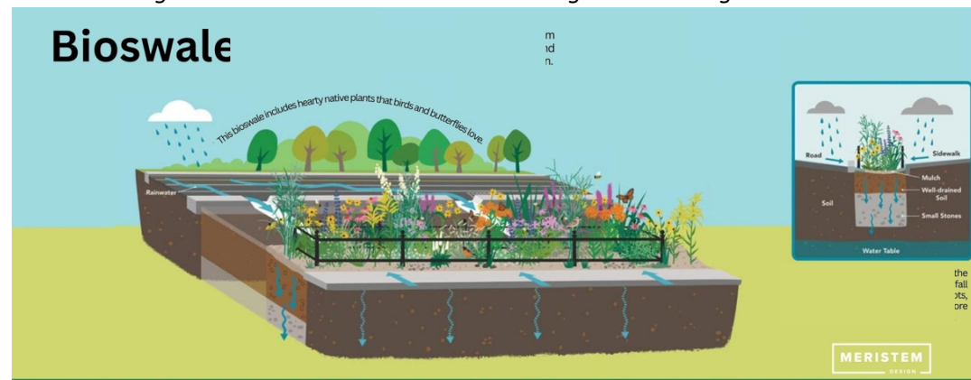
Figure 4.5 Solution to Stormwater Management Through Bioswales
